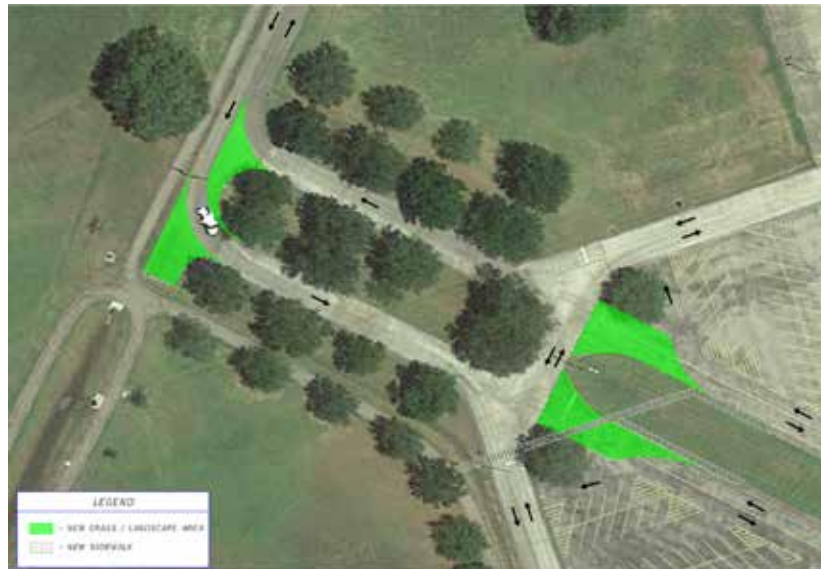
Figure 1: Reconfiguration of entrance at Childress Drive, to streamline intersection and clarify circulation paths.
